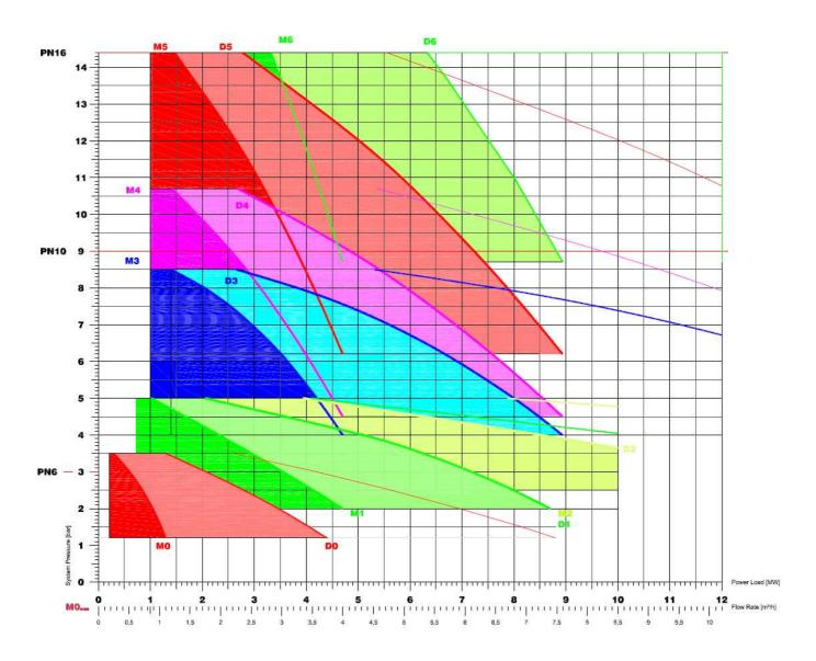
Curve designated with a prefix of 'M' show the normal characteristics of the pump module running as a single pump, curves with a prefix of 'D' show the normal characteristics of the pump module with 2 pumps running in duty assist mode.
