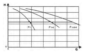
Constant pressure is maintained by the Omega ECOFlexx in a multi-pump system, in the same manner as a single pump system. The FlexxDrive can control up to four pumps to maintain constant pressure. The first pump will operate until it can no longer maintain the set pressure, then the second pump will start, followed by the third and fourth if required by the system demands.
